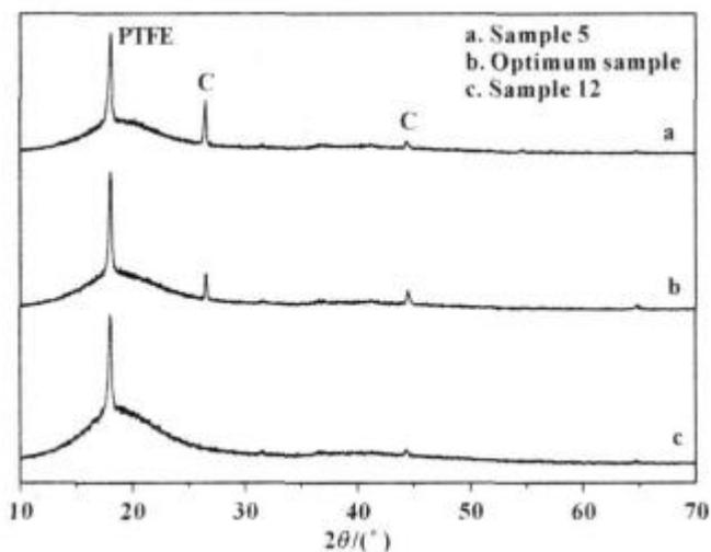
Fig.1 X-ray diffraction spectrum of epoxy resin-PTFE composite coating
