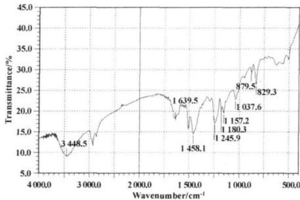
Fig.2 Infrared spectrum of epoxy resin-PTFE composite coating
