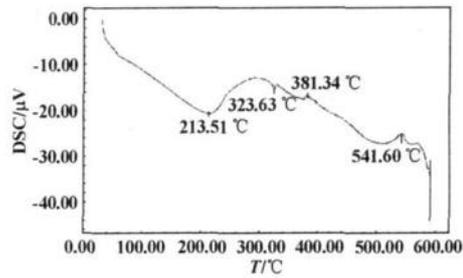
Figure 3 Differential thermal analysis of epoxy resin - PTFE composite coating
